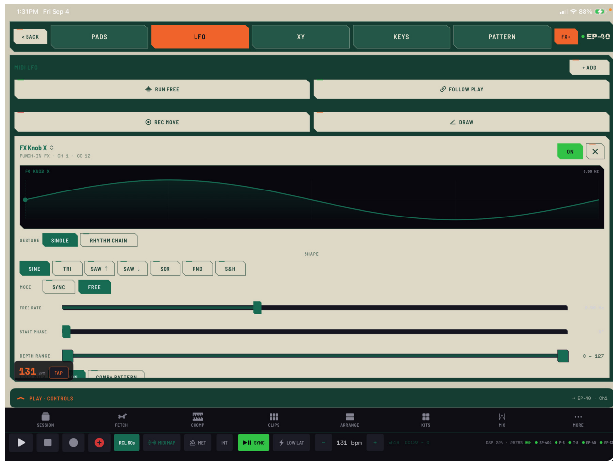
EP-40 LFO lane: shape, timing, depth and destination controls.
