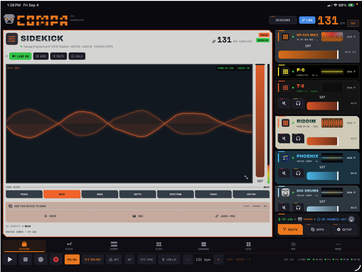
A live waveform on the Sidekick card. Scope display and control focus are separate from audio-route ownership.
