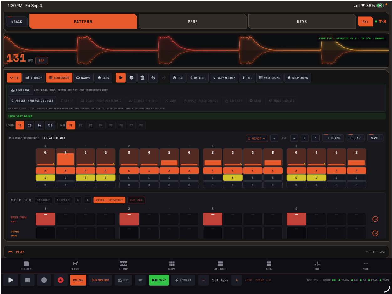
T-8 Sequencer showing the melodic lane above the drum rows. Shared beat columns and page controls keep the grid aligned; linked controls are a 1.1 (Build 30) preview.
