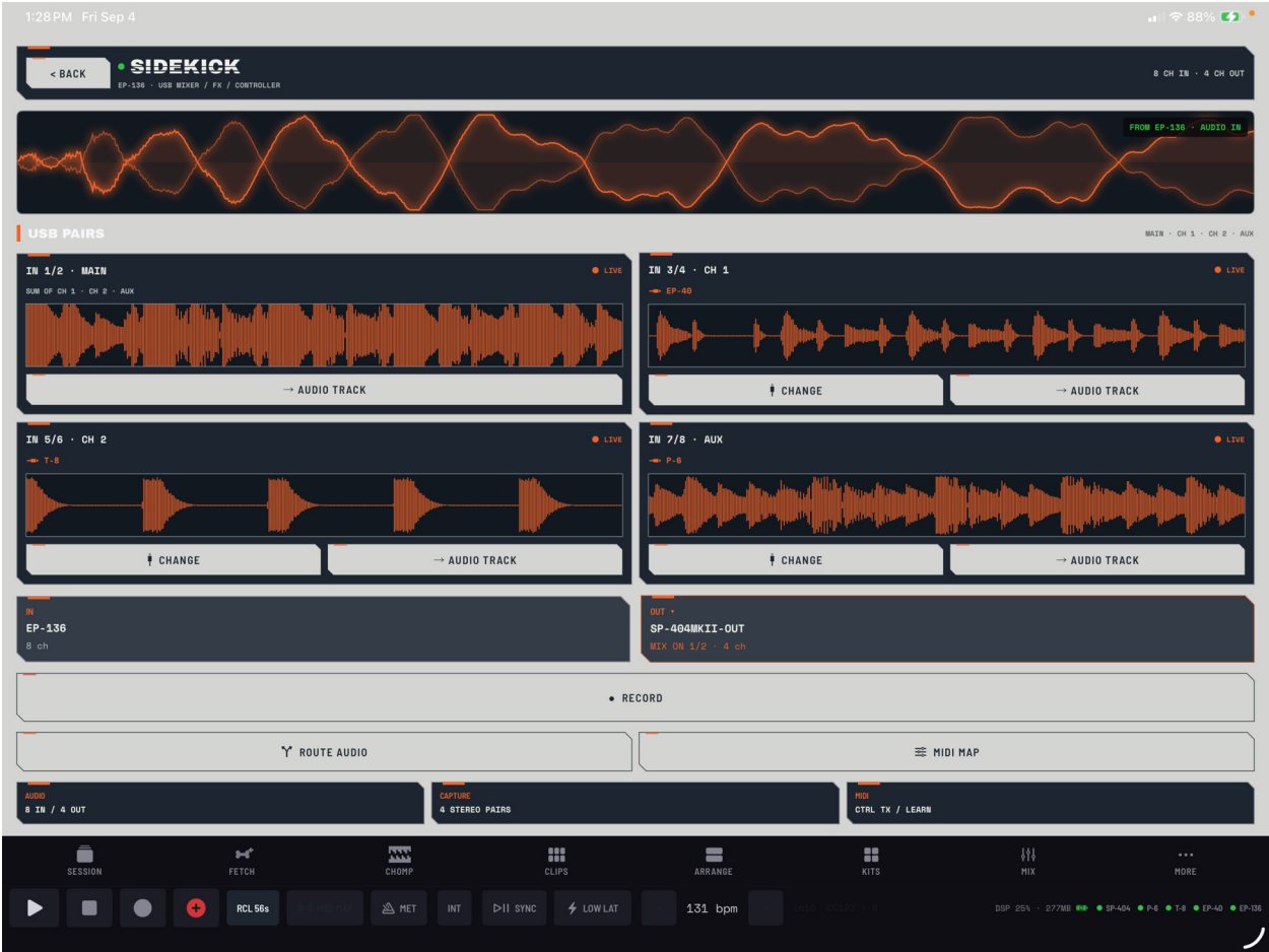
EP-136 Sidekick: physical input pairs with their own signals, names and ADD TRACK actions.
